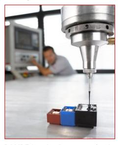
RAMPF is a leading expert for the accurate dispensing of reactive, thermally or electrically conductive polymers. The company uses its own cutting-edge dispensing systems to ensure the precise processing of these highly filled materials. The produced parts are reliably protected from contact, moisture, and damage, and thus guarantee for the lasting, high-performance functioning of electronic assemblies.
