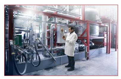
For more than 25 years, RAMPF Eco Solutions has devoted itself to the development of alternative polyols. In two of the largest facilities of their kind in Europe, tailored polyols are industrially manufactured from polyurethane residues using a specially developed chemical process.
