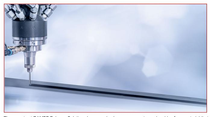
The experts at RAMPF Polymer Solutions have received numerous customer inquiries for a material that combines first-class sealing and bonding properties with the high degree of damping exhibited by elastomers. The new elastomer sealing adhesive RAKU® PUR 49-6006 Black combines all these properties into one high-performance product.
