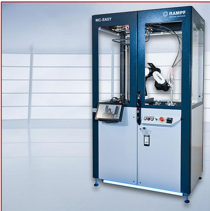
The MC-EASY Multipurpose Cell is a cost-effective solution for mixing and dispensing gap fillers and casting materials. The compact cell concept is available as a stand-alone solution but can also be effortlessly integrated into existing production lines. Thanks to its practical plug & play concept the MC-EASY allows for significant time savings both during set-up and commissioning.
