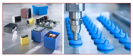
Electro casting resins based on polyurethane (RAKU® PUR), epoxy (RAKU® POX), and silicone (RAKU® SIL) offer effective and long-term protection of electrical/electronic components and ensure optimum thermal management and high thermal endurance.
