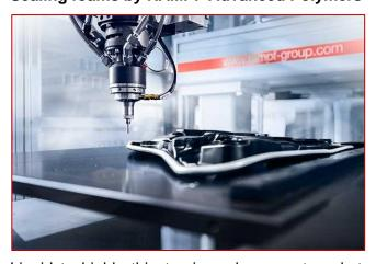
Liquid to highly thixotropic and compact gaskets based on polyurethane (RAKU® PUR) and silicone (RAKU® SIL) offer maximum long-term protection against moisture, dust, and chemicals. The high-performance products from RAMPF
