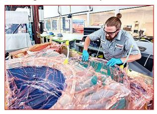
RAMPF's innovative cutting-edge Resin Infusion technology is a prime example of the company's approach to reducing its environmental impact. This method provides a sustainable alternative to traditional prepreg techniques by eliminating the need for refrigeration and autoclaves, which are known for their high energy consumption. Instead, parts are cured in lower-temperature ovens, significantly decreasing emissions compared to prepreg use.
