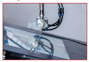
RAMPF utilizes multi-component adhesives for the precision joining of components. Pre-treatment processes enhance adhesion, and high-precision joining can be conducted manually or fully automated. Integrated curing-on-demand systems accelerate curing, and vacuum joining ensures air-bubble-free applications for products like displays (optical bonding).
