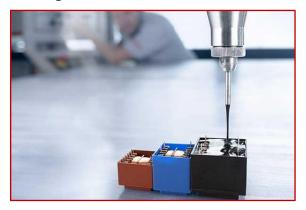
RAMPF processes reactive, thermally, and electrically conductive polymers with its premium mixing and dispensing systems, ensuring precise and fast handling of highly filled materials. The resulting parts are protected from contact, moisture, and damage, ensuring the longevity and high performance of electronic assemblies.
