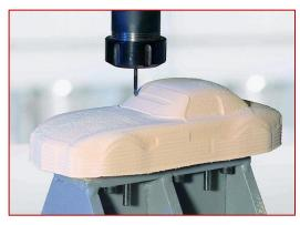
RAMPF's high-performance polyurethane board RAKU<sup>®</sup> TOOL SB-0096 is used in several industries for design studies, program proving, substructures for Close Contour paste, and negative molds for casting, amongst others. The exceptionally light board can be easily shaped, has a very good surface quality, and exhibits good resistance to heat and organic solvents.
