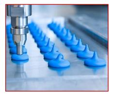
Gap fillers based on silicone (RAKU® SIL) are used in components in the battery and power electronics industries to close gaps between components and heat-dissipating surfaces. The high thermal conductivity of the thermal interface materials is increased by thinner adhesive joints and good wetting. RAMPF's low density gap filler portfolio exhibits outstanding continuous temperature resistance, aging resistance, and thixotropic properties for easy processing.
