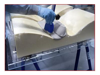
RAMPF's two-component epoxy systems are applied manually or with a CNC machine to various near net shape substructures, including RAKU<sup>®</sup> TOOL SB-0080 styling board, EPS, and cast aluminum. This significantly reduces material usage, production waste, and time for milling and finishing.
