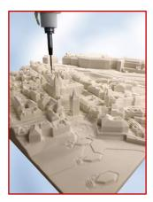
The semi-finished products – prefabricated rectangular polyurethane blocks – can be bonded to any shape and in almost any size. Customized RAKU<sup>®</sup> TOOL adhesives are available in a range of hardness levels and colors. Model-making materials are efficiently milled using CNC machines, while some boards are also suitable for manual processing.
