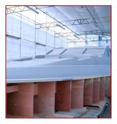
The innovative two-component epoxy systems are applied to nearcontour substructures using mixing and dispensing systems, either manually or with a CNC machine. Compatible with a wide range of substructures – including RAKU<sup>®</sup> TOOL styling block SB-0080 and EPS – Close Contour Pastes cure quickly at room temperature before milling according to CAD data.
