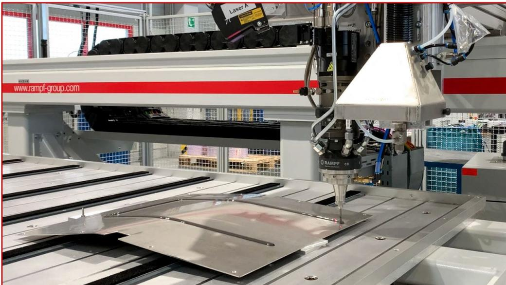
Even on an unpainted, high-gloss surface, the polyurethane sealing foam is applied seamlessly. In addition to the two-component mixing head with distance control, the system is equipped with a fully automatic primer application nozzle with integrated suction.
