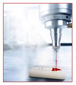
Climbing hold manufacturers with higher volumes benefit from RAMPF's contract manufacturing services. The company uses proprietary, automated mixing and dispensing systems for the fast, cost-efficient, and flexible manufacture of high-performance climbing holds at its facility in Suwanee, GA.
